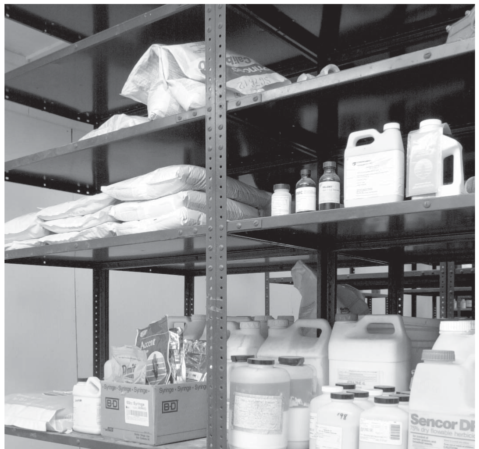
Figure 4. Metal shelving is used to store dry pesticides above liquid pesticides.
